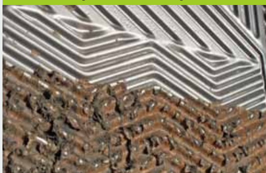
Plate Heat exchanger - before/after cleaning
